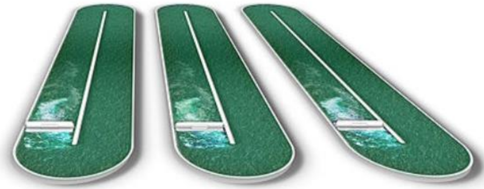
Figure 3: Typical RAP as endless loop with water moved by electrically driven paddle wheel. Depth of roughly 20-30 centimeters ( www.wikiwand.com/en/Algae_fuel )
