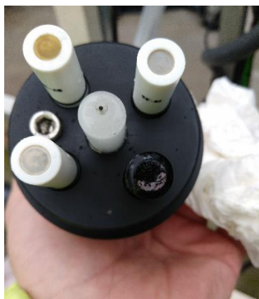
Ammonia/Nitrate sensor. Reference electrode in the centre, where a black spot can be seen due to fouling.
