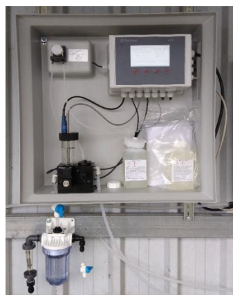
Detail of the phosphate analyser.
